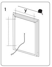
Measure the distance between the two ends, this mirror can be hung horizontal or vertical.
