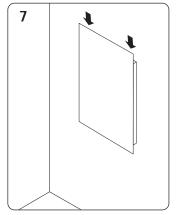
Slide the mirror down onto the screws, check if secure.
