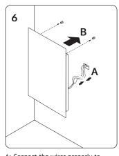
A: Connect the wires properly to their corresponding colour.
