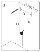
Using a pencil and a level, mark the desired position on the wall.
