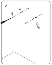
A: Insert wall plugs B: Insert screws
