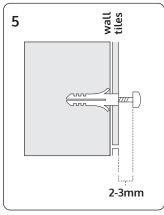
Leave a 2-3mm gap between the screwhead and wall.
