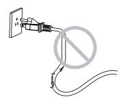
The power socket in use should be within the specified range (AC120V). ※Risk of fire and/or electric shock.
